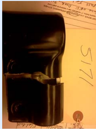
Broken upper Hinge assembly
